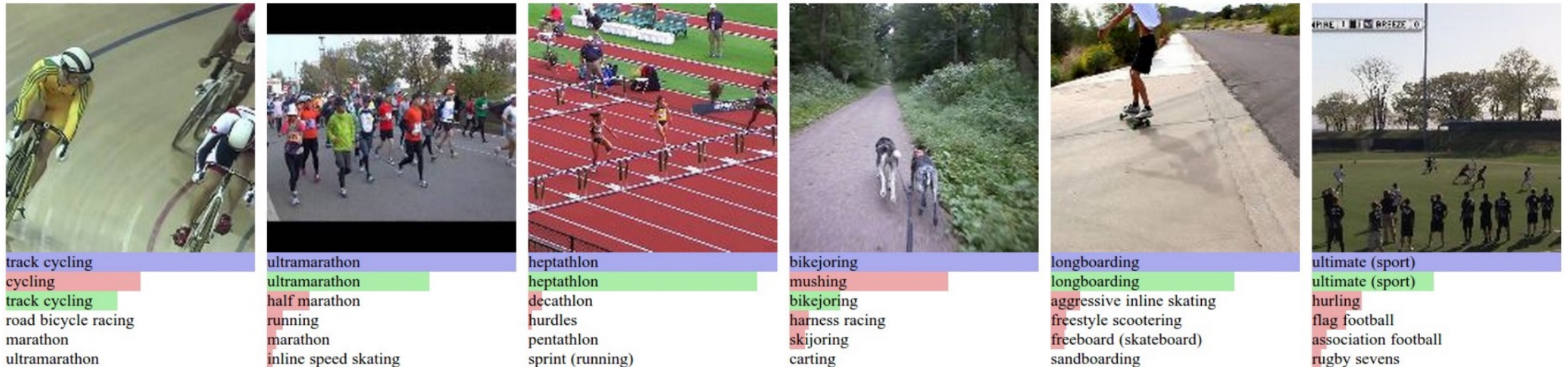
Figure 4: Predictions on Sports-1M test data. Blue (first row) indicates ground truth label and the bars below show model predictions sorted in decreasing confidence. Green and red distinguish correct and incorrect predictions, respectively.
